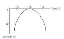
To calculate the frequency stability the parabolic curvature constant (K) is needed. For calculating the stability at 45°C? 1- Change in temperature ( $\Delta$ T) is (45-25) = +20°C 2- Change in frequency is (-0.034 x ( $\Delta$ °C)²) = (-0.035 x (20)² = -13.6ppm
